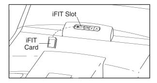
Next, select an iFIT workout by pressing the iFIT up and down buttons next to the iFIT slot. When an iFIT workout is selected, the display will show the name of the workout, duration, the maximum incline setting, and the maximum speed setting of the workout. In addition, a profile of the speed settings of the workout will appear in the display.
